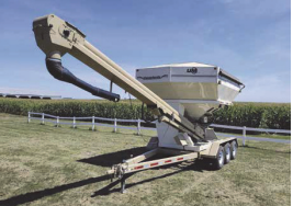
*Unverferth Seed Runner 3750XL Self Filling Seed Tender, Scale, Roll Tarp, Lights, Honda GX390 Engine with Electric Start, Tri Axle with ST235/85R16 Tires, SN: D60870153
